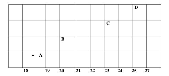
A is identified as Easting 18 and northing 41. The four grid reference is 1941 The six grid reference is 194 419.
